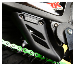
2 x Bolts & Washers M6x20 - 10Nm
