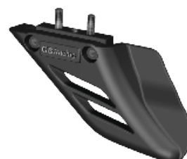
2 x Bolts & Washers M6x20 - 10Nm
