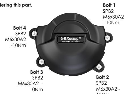
**SECONDARY ALTERNATOR & OIL PRESSURE SENSOR COVER – PART NO. EC-R6-2017-1-GBR**
