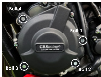
Bolt 3 SPB-9 M6X50HHF - 10Nm
