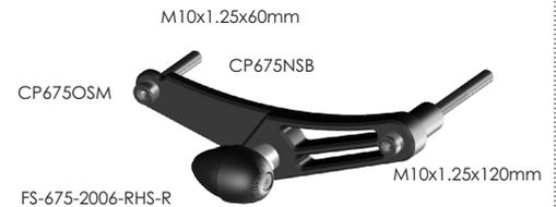
3. Assemble black anodised bracket. Use 1 off M10 x 120 x 1.25 & 1 off M10 x 60 x 1.25 nickel plated bolts. Re-use the original M10 locking nut.
