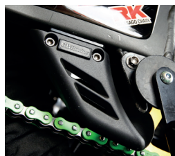
2 x Bolts & Washers M6x20 - 10Nm
